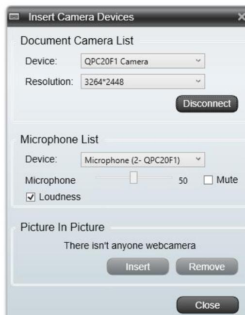
Select the device (ex: “QPC20F1 Camera”) or other connected camera device, and select the resolution from the drop-down list (the resolutions displayed here depends on the camera you are using)
