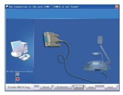
When the indicator of "Current RS-232 Connection Status" is green, that means the connection between the visualizer and the computer's RS232 connector is good. If the indicator is red, please check if the RS232 cable is connected correctly. When all the cables are connected correctly, please click
