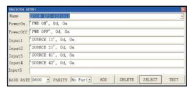
Connect the visualizer to a computer with a RS232 cable (Please disconnect the projector from the RS232 port first) and select the Baud Rate and Parity based on the projector's Baud Rate, then click the "TEST" button to pop up the Projector Code Test dialog box, input the Baud Rate and Parity based on the projector's Baud rate, then click
