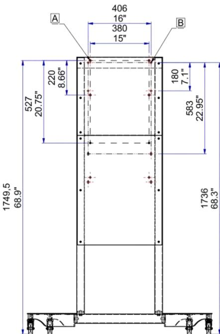
**A:** The Mobile Stand Mix® has 2 mounting positions for the BalanceBox® 400 or the Universal VESA Bracket:
