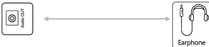
◆Note: Audio-OUT port can be connected with a headset or an external speaker.
