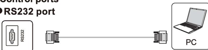
◆Note: RS232-IN port is connected to the PC; the product is operated via the PC.
