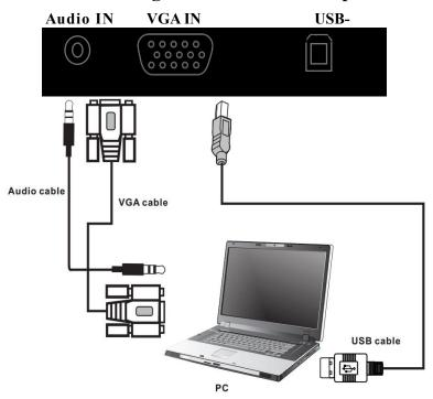
Connect your computer using a USB touch cable, VGA Cable and Audio Cable, HDMI Cable or DP Cable.
