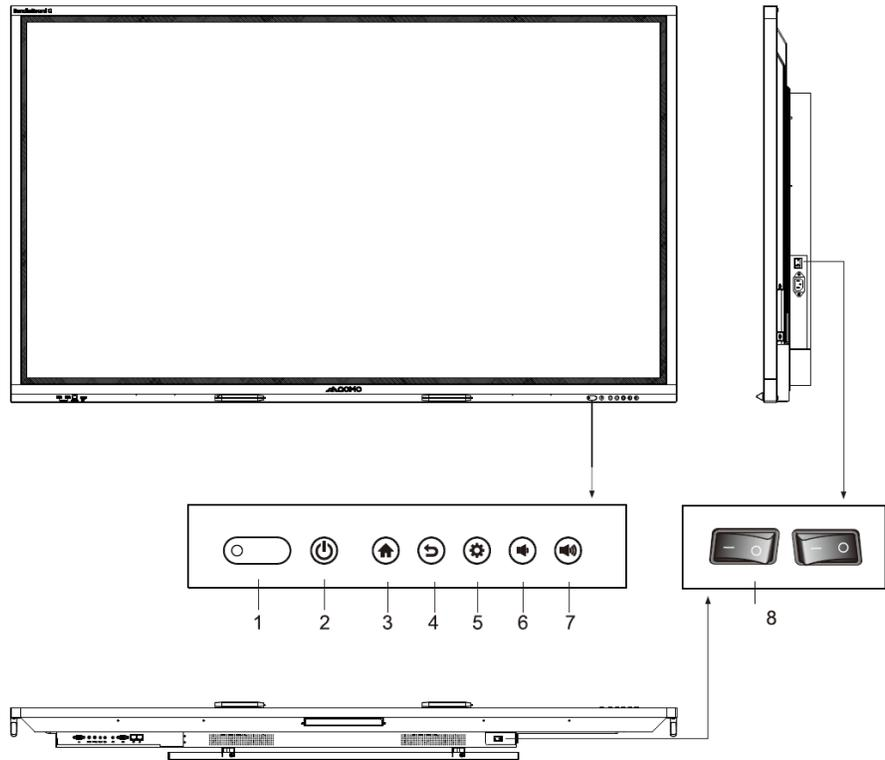
1. Indicator light, remote control receiver and light sensing receiver;
