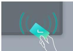
After the device powers on, swipe the designated user's NFC card over the reader. The system will automatically switch to the associated user account and unlock the screen.
