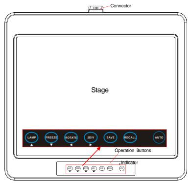
If the unit come with a light box, to connect it to the unit, turn on the backlight by pressing the "LAMP" key, and then press the "NEG" button on the Remote Control to display the film negatives. There are some buttons on the light box ,you can also control the unit by these buttons.
