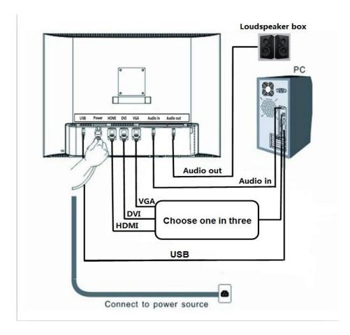
(1) Connect the HDMI cable to the HDMI input port on the side of the QIT600F1, and tighten the screws to fasten. Connect the other end of the cable to the PC HDMI port, and tighten the screws to fasten.
