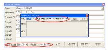
Click the projector control buttons on the visualizer's operating panel to check if the control code that the program received is the same as the sending code. If the receiving code is same to the sending code, the input codes are correct. If the visualizer can not control the projector, please do the following.
