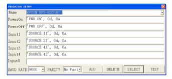
The input format of projector's control code is as follows:
