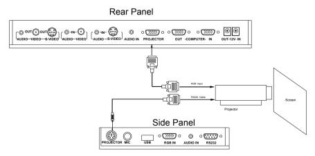
Connect the PROJECTOR port to the projector's RGB IN port using the
