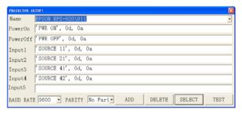
Connect the visualizer to a computer with a RS232 cable (Please disconnect the projector from the RS232 port first) and select the Baud Rate and Parity based on the projector's Baud Rate, then click the "TEST" button to pop up the Projector Code Test dialog box, input the Baud Rate and Parity based on the projector's Baud rate, then click "Open".
