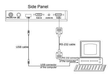
Use the computer RS232 cable (9-pin to 9-pin) to make the
