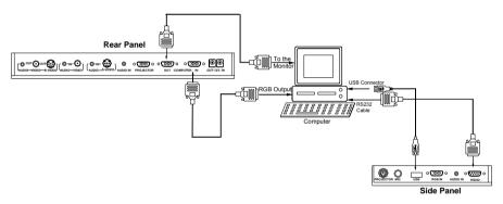
**Note:** You can connect a laptop computer to the RGB IN port of side panel using a RGB cable.
