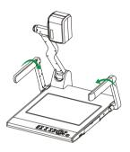
Carefully fold the camera stand down to the front panel
