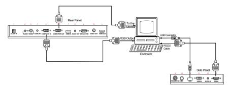
**Note:** You can connect a laptop computer to the RGB IN port of side panel using a RGB cable.
