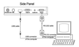
Use the computer RS232 cable (9-pin to 9-pin) to make the connections displayed below to control the visualizer from an external computer. A USB connection e nables the computer to capture still images an d/or video streams from the visualizer . Special software is r equired for this operation.
