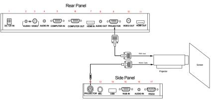
Connect the PROJECTOR port to the projector 's RGB IN port using the RGB cable. You can also control a projector using the controls on the visualizer by connecting the projector to the visualizer using a 6-pin to 9-pin
