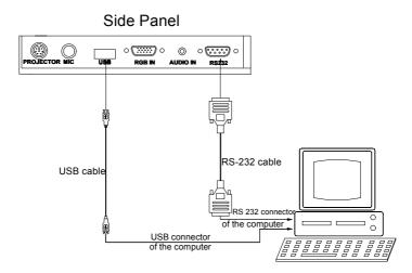
Use the computer RS232 cable (9-pin to 9-pin) to make the connections displayed below to control the visualizer from an external computer. A USB connection enables the computer to capture still images and/or
