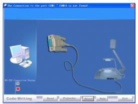
When the indicator of "Current RS-232 Connection Status" is green, that means the connection between the visualizer and the computer's RS232 connector is good. If the indicator is red, please check if the RS232 cable is connected correctly. When all the cables are connected correctly, please click "Projector" to select your projector model under the drop-down list, then click "Send". If you can not find your particular projector model in the "Projector", please do the following:
