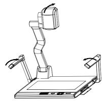
2. Carefully **fold** the camera stand down to the front panel.
