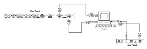
Step 4: Connect to the first video equipment with S-Video input.
